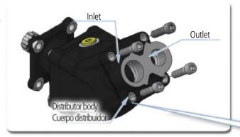
To change the direction of rotation remove the 4 screws and, keeping the distributor body close to the pump, rotate it by 180°.
